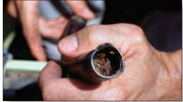
Fig. 5.27 It is critical to check drills thoroughly before use. Not only must the drill be calibrated before planting (according to PLS estimation), but general maintenance is also required. This drill wasn't planting switchgrass. Why? The drop tubes coming out of the small seed box were clogged. Drop tubes, chain sprockets, seed boxes and grease fittings all need attention before planting.
