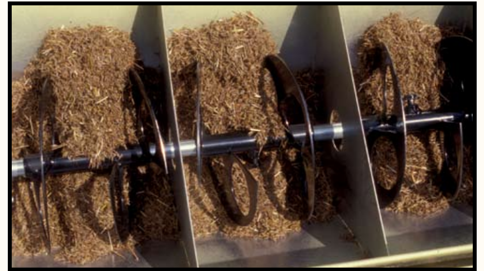
Advancements in planting technology, such as this native grass seed box on a Truax drill, and herbicide development have made establishing native grasses and forbs relatively easy.
